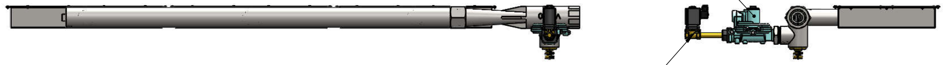
[6213-050-230VAC] SOLENOID VALVE 2/2, SIZE 1/2" COIL 230V/50Hz - ORIFICE 13MM "BURKERT"
